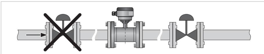
Figure 3-11: Installation in front of a control valve
