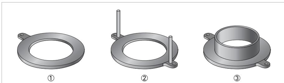
Figure 4-2: Different types of grounding rings
