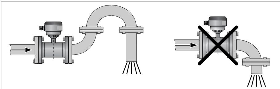
Figure 3-10: Installation in front of an open discharge
