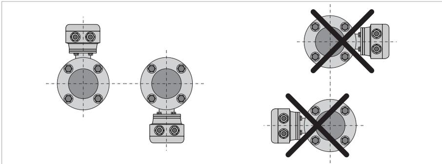
Figure 3-3: Mounting position
