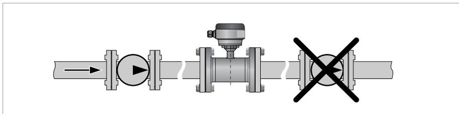
Figure 3-13: Installation behind a pump
