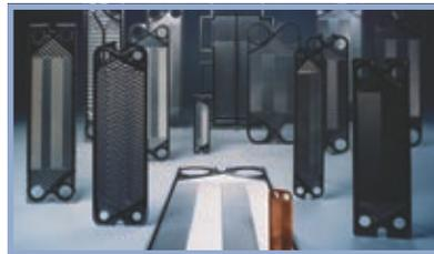
The Schmidt line of gasketed plate & frame heat exchangers provide excellent heat transfer in a compact space. Plates are pressed from stainless steel, titanium and other alloys. Gaskets of nitrile, EPDM, Viton®, compressed fiber and Teflon® are used. Capacities range from 0.5 to 10,000 GPM.
