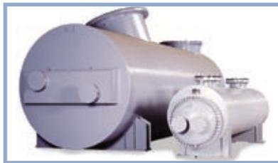
Unique, patented plate-fin design for centrifugal or axial compressor intercooler and aftercooler applications and minimal pressure loss. Design eliminates separators. ASME code design is standard. Diameters from 20" (50.8 cm) to 120" (304.8 cm).
