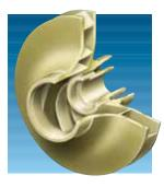
Precision Cast Closed Impeller is statically and hydraulically balanced to reduce power consumption. The impeller is keyed to shaft to provide positive drive and eliminate impeller spin-off. Balancing holes through the impeller hub minimize axial thrust and seal chamber pressure.
